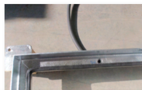
In the deck frame there is an installation hole for a drain hose for water that leaks in to the frame. It is used especially for outdoor installation.
